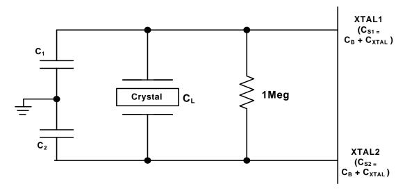
Figure 6.1 Typical Crystal Circuit
